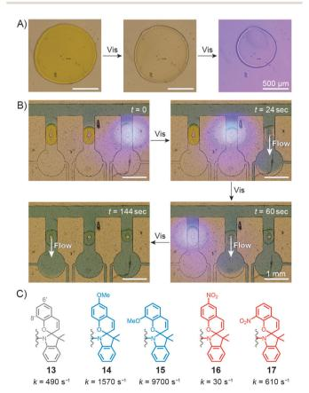
Fig. 10 Spiropyran-based microvalves. (A) Contraction of a poly(NIPAM-SP) gel induced by blue light. (B) Remote control of liquid flow by consecutive opening of poly(NIPAM-SP)-based microvalves using blue light. (C) Controlling the rate of SP ring closure by the substitution pattern on the chromene moiety. [Adapted with permission from ref. 231 (Copyright 2007 Elsevier) (A and B).]
