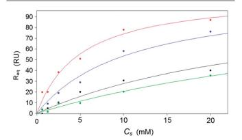
**Fig. 4** Calibration curve of control subtracted SPR response change for *bis*-BA sensor *versus* glucose (red), fructose (blue), galactose (black) and mannose (green) (0.3 mM, 0.6 mM, 1.25 mM, 2.5 mM, 5 mM, 10 mM and 20 mM).
