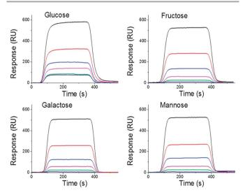
**Fig. 3** SPR kinetic measurements showing the binding of p-glucose, p-galactose, p-fructose and p-mannose to 1 : 1 *bis*-BA : TEGT SAMs using different saccharides concentrations (0.6 mM, 1.25 mM, 2.5 mM, 5 mM, 10 mM and 20 mM).
