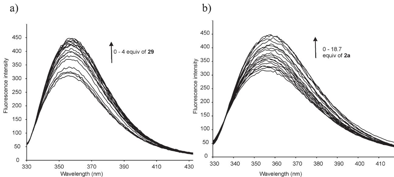
**Fig. 7** Fluorescence titration of receptor **26** with  $\alpha$ -maltoside **29** (a) and  $\beta$ -glucopyranoside **2a** (b) in  $\text{CHCl}_3$ ;  $[\mathbf{26}] = 8.51 \times 10^{-5}$  and  $9.57 \times 10^{-5}$  M; Equiv. of **29** = 0.00–4.03; Equiv. of **2a** = 0.00–18.69. Excitation wavelength 324 nm. Fluorescence intensity increased with increasing sugar concentration.<sup>24</sup>
