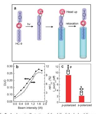
**Fig. 8** A schematic illustration of the shift of the hydrophilic part (red) to the very end of the head part in the photoexcited state, and the subsequent insertion into silicalite-1 channels with the tail part first (a). Plots of the DUO and rel- $I_{2\omega}$  (in %) with respect to the laser beam intensity (b) and the effect of the beam polarization direction (p or s) on the  $I_{2\omega}$  (on) to  $I_{2\omega}$  (off) ratio (c). (Adopted from ref. 48.)
