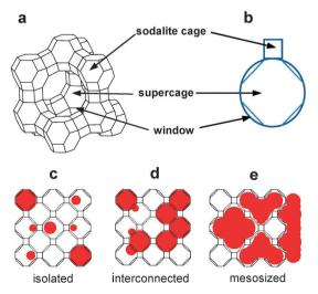
Fig. 12 Structures of zeolite Y, its cages, their geometrical representations, and illustration of three types of QDs.
