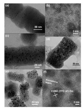
**Fig. 3** Ex situ TEM images of nanodisks after the 1st cycle (a and b), after 50 cycles (c), after 100 cycles (d) and after 220 cycles (e and f); (f) is an expanded image of (e).
