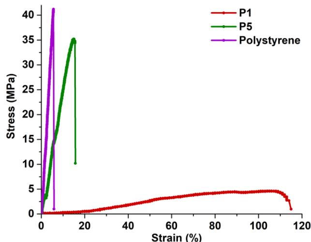
**Figure 5.** Tensile properties of polymers. Representative stress–strain curves of P1, P5, and commercial polystyrene at room temperature.
