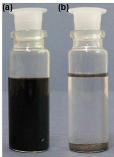
**Fig.1** Photograph showing the formation of Mn-Al colloidal nanoparticles (suspension) in the case of 8-h milled Mn-Al powders with OA+OY (a), which is compared with that of those prepared without OA+OY (b).
