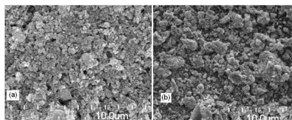
**Figure 3** SEM images of  $CuFe_2O_4$  nanoparticles before (a) and after (b) 3<sup>th</sup> cycle.
