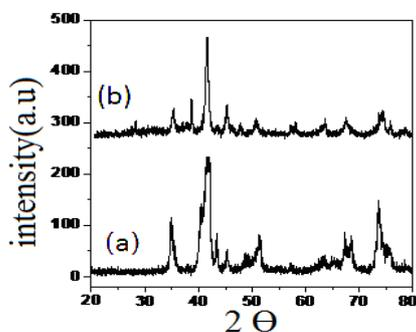
**Figure 1** (a) XRD spectrum of native  $CuFe_2O_4$  catalyst. (b) XRD spectrum of reused  $CuFe_2O_4$  catalyst after 3<sup>th</sup> cycle.
