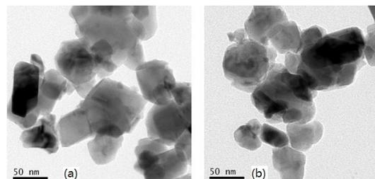
**Figure 2.** (a) TEM image of the fresh  $CuFe_2O_4$  nanoparticles. (b) TEM image of the  $CuFe_2O_4$  nanoparticles after 3<sup>th</sup> cycle.
