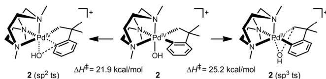
**Scheme 4** Calculated activation parameters for C(sp<sup>2</sup>)-O vs. C(sp<sup>3</sup>)-O bond formation reactivity of **2**.
