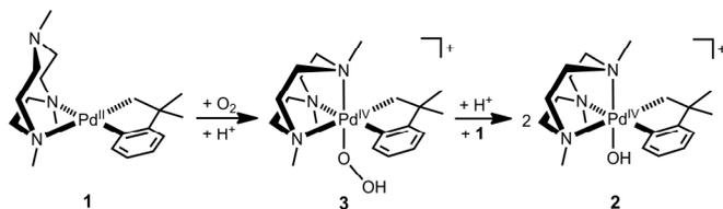
Scheme 2 Proposed mechanism for aerobic oxidation of **1**.
