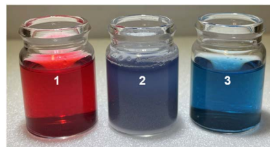
Fig. 10 Samples of red cabbage extract prepared according to the method described by James Watt. Sample 1 shows cabbage extract in dilute \text{H}_2\text{SO}_4 , sample 2 shows cabbage extract mixed with \text{CaCO}_3 (unfiltered) and sample 3 shows extract mixed with \text{CaCO}_3 and resulting \text{CaSO}_4 has been filtered off.
