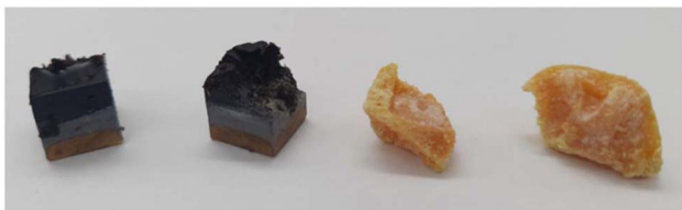
Fig. 9 Inverse vulcanised polymers showing visual evidence of the sulfur bloom effect. The polymers on the right show severe sulfur bloom all over the pieces due to being made with excessively high sulfur contents and not being cured. The polymers on the left show moderate sulfur bloom. Note how the sulfur bloom occurs toward the bottom of these polymer cubes because they were poured into a 1 cm 3 mould too early in their reaction, resulting in the denser sulfur sinking to the bottom of the cube in the absence of stirring. This led to excessively high sulfur concentrations in the bottom of the cube in comparison to the top, which could not be stabilised, resulting in sulfur bloom. Reproduced with permission from RSC Appl. Polym. , 2025, 3, 10–42. Under the Creative Commons Attribution 3.0 Unported Licence, Royal Society of Chemistry.
