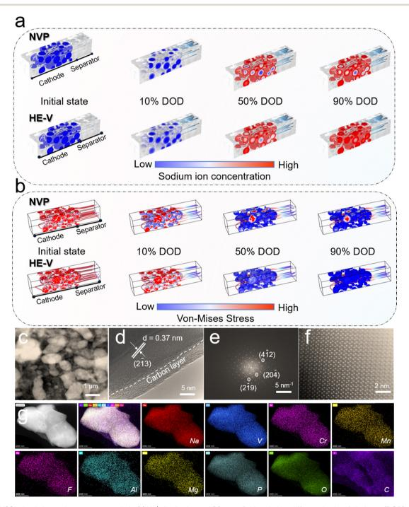
Fig. 5 COMSOL simulation and postmortem analysis. (a) Na<sup>+</sup> distribution and (b) stress field analysis at different depths of discharge (DOD) states based on the COMSOL platform. Postmortem analysis of the cycled HE-V: (c) TEM, (d) HRTEM, (e) FFT, and (f) aberration-corrected STEM image. (g) EDS mapping images
