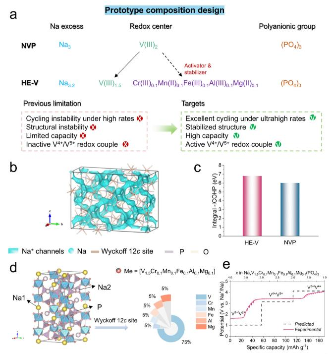
Fig. 1 Composition design principle and theoretical studies of physicochemical properties. (a) Prototype composition design principle. (b) Na<sup>+</sup> ion diffusion pathways (blue isosurface) in HE-V from the BV calculation. (c) Integral ICOHP values of all V-O bonds in HE-V and NVP. (d) Illustrations of crystalline structures and transition metal compositions in HE-V. (e) Calculated voltage profile.
