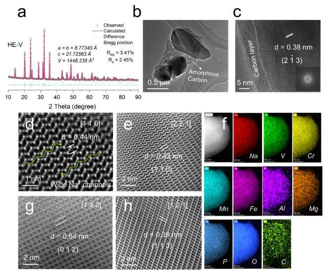
Fig. 2 Material characterization of HE-V. (a) XRD Rietveld refinement results. (b) and (c) TEM and HRTEM images. (d)-(h) Aberration-corrected STEM images viewed from the (d) [110], (e) [221], (g) [142], and (h) [121] crystallographic directions. (f) EDS mapping images (scale bar: 50 nm).
