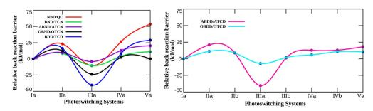
Fig. 4 Variation in the barrier for thermal back isomerization of the photoproduct to bicyclodiene in various N-substituted systems relative to that of their parent photoswitching system. The energy values were obtained by computing the electronic energy with the (8,8)-CASPT2/6-311++G\*\* level of theory
