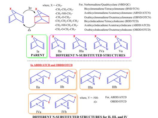
in ABDD/ATCD and OBDD/OTCD Scheme 1 Schematic representation of the various parents and N-substituted bicyclodiene based photoswitching systems considered for the study.
