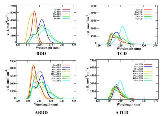
Optical absorption spectra of the parent and N-substituted BDD/TCD and ABDD/ATCD photoswitching systems
