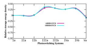
Fig. 3 Variation in the energy storage density of N-substituted systems relative to that of their parent photoswitching system. The energy values were obtained by computing the electronic energy with the DLPNO-CCSD(T)/Def2TZVP method and including thermal correction at the M062X/6-311++G\*\* level.
