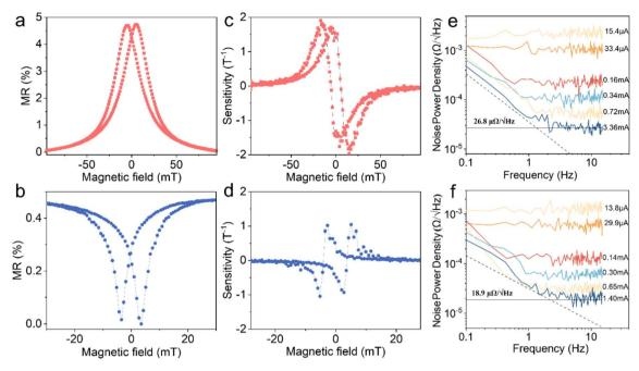
Fig. 2 Magnetoelectric performance of printed magnetoresistive sensors. (a) MR, (c) sensitivity and (e) noise of the printed sensor with  $[Co/Cu]_{50}$  GMR microflakes as functional fillers. (b) MR, (d) sensitivity and (f) noise of the printed sensor with  $Ni_{97}Co_3$  AMR microparticles as functional fillers. All measurements are performed at room temperature.
