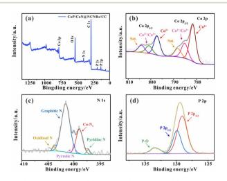
Fig. 3 (a) XPS spectrum, (b) Co 2p, (c) N 1s, and (d) P 2p of CoP/CoN@NCNRs/CC.
