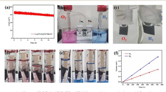
Fig. 9 (a) Long-term durability test of CoP/CoN@NCNRs/CC at 1.65 V, (b) water splitting assembly diagram, (c) O2 and H2 generation from the anode and cathode, (d and e) linearity of O2 and H2 production over time, and (f) oxygen and hydrogen generated at 0, 3, 6, 9, and 12 min.
