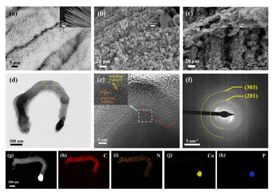
Fig. 2 (a) SEM images of  $Co(CO_3)_xOH_y/CC$  nanoneedle arrays. Inset: details of the nanoneedle arrays, (b) SEM of Co@NCNRs/CC and the inset shows the details of single Co@NCNR, and (c) SEM of CoP/CoN@NCNRs/CC; (d) TEM and (e) HR-TEM. Inset: lattice spacing of CoP and CoN, (f) SAED pattern, and (g-k) compositional elemental mapping of CoP/CoN@NCNRs/CC.
