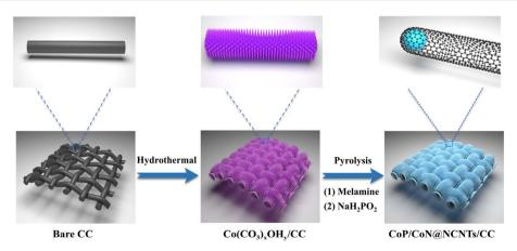
Scheme 1 Illustration for the fabrication of CoP/CoN@NCNRs/CC.
