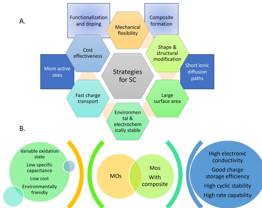
Fig. 6 (a) Enacted strategies to improve the performance of electrode materials for high-energy supercapacitors. (b) Characteristics of metal oxides and metal oxide composites in SC.
