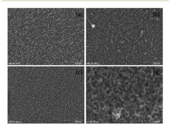
Fig. 3 SEM images of various samples grown at (a) 800  $^{\circ}$ C on silicon (b) 800  $^{\circ}$ C on quartz (c) and (d) 500  $^{\circ}$ C on quartz.
