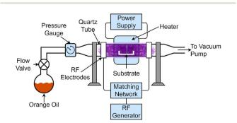
Fig. 1 PECVD apparatus utilized in this work.
