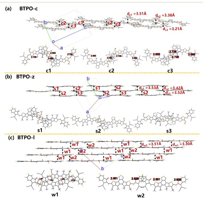
Fig. 7 The single-crystal packing diagrams of (a) BTPO-c, (b) BTPO-z and (c) BTPO-l along the  $\pi-\pi$  stacking direction with the corresponding dimer structures. Here, all the side chains are simplified with methyl or methoxy for clarity.
