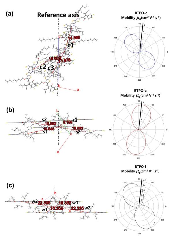
Fig. 8 (a–c) Molecular packing viewed along the normal to the plane of interest (left: the number in green stands for the hoping distance (r, Å)) and corresponding simulated anisotropic electron mobility curves based on the hopping model (right) of (a) BTPO-c, (b) BTPO-z and (c) BTPO-l.
