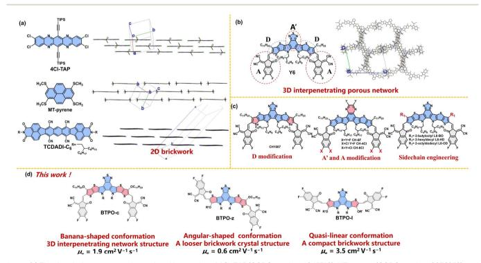
Fig. 1 (a) The chemical structures and crystal packing modes of 4Cl-TAP (CCDC number: 1845318), MT-pyrene (CCDC number: 2076078), and  $TCDADI-C_6$  (CCDC number: 2255617). (b) The chemical structures and crystal packing modes of the most famous BTP derivative Y6 (CCDC number: 2015912). The long alkyl chains are simplified with methyl or isopropyl and the hydrogen atoms are omitted for clarity. (c) Design strategies and chemical structures of BTPO-t in this work.
