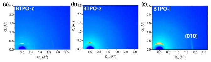
2D-GIWAXS patterns: BTPO-c film (a), BTPO-z film (b), and BTPO-l film (c).
