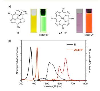
Fig. 4 (a) Photographs of  $CH_2Cl_2$  solutions of **8** and ZnTPP under room light and UV light. (b) UV-vis absorption (solid line) and emission (dashed line) spectra of subporphyrin **8** and tetraphenylporphyrin (ZnTPP) in  $CH_2Cl_2$ .
