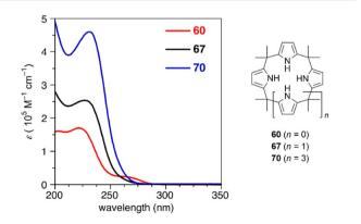
Fig. 6 UV-vis absorption spectra of calix[n] pyrroles (n=3, 4, 6) in acetonitrile.
