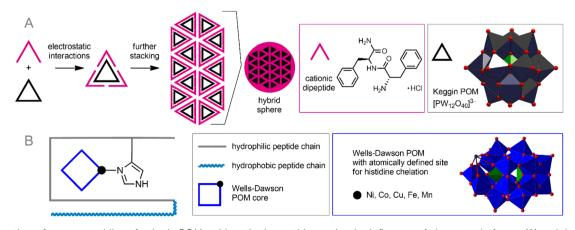
Fig. 3 Formation of nanoassemblies of anionic POMs with cationic peptides under the influence of electrostatic forces (A) and the synergetic effect of coordination bonds and electrostatic forces (B).
