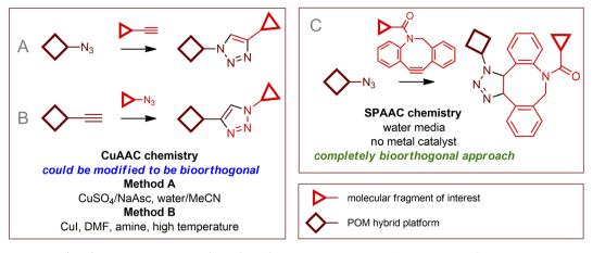
Fig. 6 Click chemistry for (post)functionalization of POMs: CuAAC conjugation of azide-functionalized POM to terminal acetylene (A); CuAAC conjugation of POM bearing a terminal acetylene group to azide (B); SPAAC conjugation of azide-functionalized POM to a 3'-dibenzocy-clooctyne-derived building block (C).
