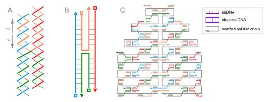
Fig. 10 DNA crossover between helices: helix representation (A); base pairing and schematic line representation showing antiparallel base pairing with 5' and 3' ends denoted by squares and triangles, respectively (B); DNA origami structure involving scaffold ssDNA strand (black line) and multiple short staple ssDNA strands (colored lines) (C).
