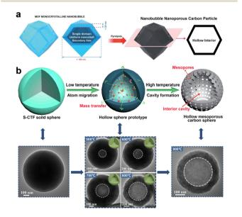
Fig. 5 (a) Preparation of nanobubble carbon via the pyrolysis of MOF nanobubbles. Reproduced with permission from ref. 85. Copyright 2017, Royal Society of Chemistry. (b) The fabrication process of N, S co-doped hollow mesoporous carbon sphere (N/S-HMCS) and the corresponding TEM images. S-CTF represents the sulfur-bridged covalent triazine frameworks. Reproduced with permission from ref. 89. Copyright 2021, Elsevier.
