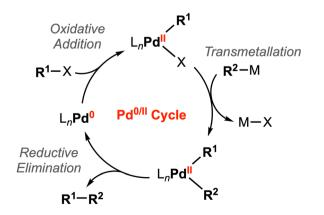
Fig. 3 General catalytic cycle for Pd-catalyzed reactions.16
