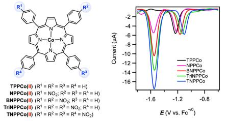
Fig. 12 Cobalt(II) tetraphenylporphyrin complexes and their differential pulse voltammograms in DMF with 0.1 M ["Bu<sub>4</sub>N][PF<sub>6</sub>]. Reproduced from ref. 66 under a Creative Commons License CC-BY-NC-ND 4.0.
