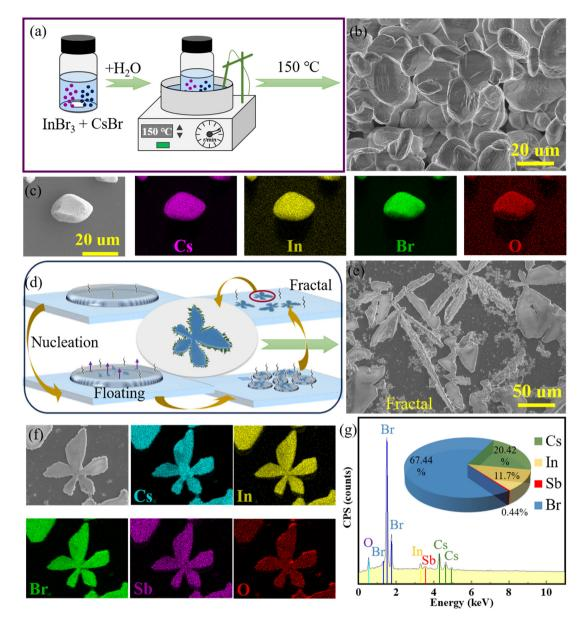
Fig. 1 (a) Preparation process of  $Cs_2lnBr_5(H_2O)$ ; (b) SEM image of  $Cs_2lnBr_5(H_2O)$  prepared at 150 °C; (c) EDX mapping of Cs, In, Br, and O elements; (d) fractal structure of  $Cs_2ln_{1-x}Sb_xBr_5(H_2O)$  samples obtained *via* the *in situ* solution crystallization method; (e) SEM image of the fractal structure post-crystallization; the EDX mapping (f) and EDX spectrum (g) of  $Cs_2lnBr_5(H_2O)$ :Sb.
