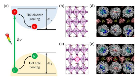
Fig. 1 Schematic illustration of hot carrier relaxation (a). Optimized ground state structures of pristine MAPbI<sub>3</sub> (b) and MAPbI<sub>3</sub> with Pb<sub>V</sub> (c). Superimposed snapshots of local structures from 5 ps molecular dynamics trajectories of pristine (d) and defective (e) MAPbI<sub>3</sub>. The red dashed circle denotes the location of vacancy site. The motion of MA cations in the defective system is enhanced due to the additional space created by Pb vacancies.
