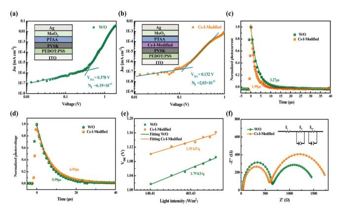
Fig. 5 Dark J-V curves of the hole-only devices with the structures of (a) ITO/PEDOT:PSS/Perovskite/PTAA/MoO<sub>3</sub>/Ag and (b) ITO/PEDOT:PSS/Cs-I-modified Perovskite/PTAA/MoO<sub>3</sub>/Ag. (c) TPC and (d) TPV decay curves, (e) V<sub>OC</sub> as a function of light intensities, and (f) Nyquist plots of the PSCs without and with Cs-I modification
