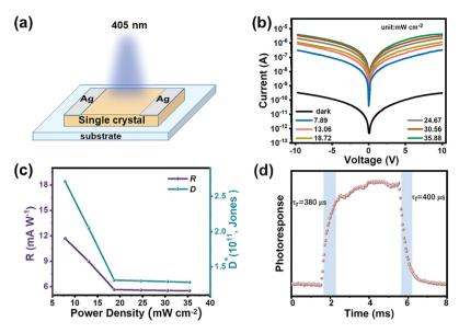
Fig. 4 (a) The photodetection device schematic diagram of 1. (b) The I-V curves of 1 measured at 405 nm with different incidence powers. (c) R and D\* calculated from the photocurrent measured at 10 V bias. (d) The response time of 1.
