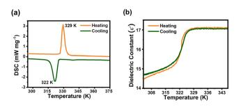
Fig. 2 (a) The DSC curve of  ${\bf 1}$  and (b) the dielectric constant curve of  ${\bf 1}$  at 1000 kHz.
