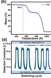
Fig. 5 (a) The phase stability of 1 by the PXRD patterns. (b) TG curve of 1. (c) The photoresponse capability of 1 after 800 and 1200 I-T cycles at 405 nm. (d) Periodic of repeatable switching measurement after several on/off cycles at 1 MHz.
