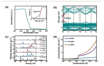
Fig. 3 (a) The UV-vis absorption spectrum of 1 (inset: the experimental bandgap). (b) The calculated bandgap diagram of 1. (c) PDOS of 1. (d) Variable temperature conductivity test along different axes of single crystals.
