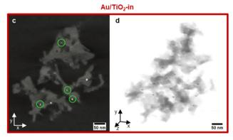
Fig. 3 3D analysis of the NP placement using electron tomography. XY-slices taken from the 3D reconstruction showing the interior of the 5 wt% (a) Au/TiO<sub>2</sub>-on and 3 wt% (c) Au/TiO<sub>2</sub>-in IO films and the corresponding 3D XYZ views in (b and d). Au NPs are shown as bright white spots in (a and c) and dark spots in (b and d). The green circles in (c) indicate embedded Au NPs.
