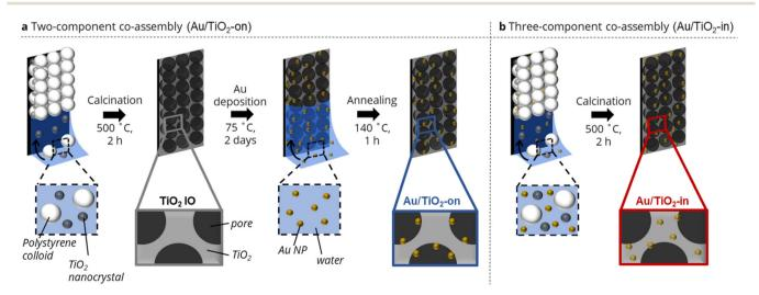
Fig. 1 Schematic illustration of Au/TiO<sub>2</sub> IO film synthesis in which Au NPs are placed either (a) on the TiO<sub>2</sub> surface via a two-component co-assembly approach, or (b) in the TiO<sub>2</sub> matrix via a three-component co-assembly approach.
