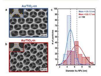
Fig. 2 Structural characterization of  $Au/TiO_2$  IO films. SEM images of 5 wt% (a)  $Au/TiO_2$ -on and 3 wt% (b)  $Au/TiO_2$ -in. Au NPs are shown as bright white spots. Inset schematically depicts the expected Au NP placement in the  $TiO_2$  IO film. (c) Au NP size distribution in  $Au/TiO_2$  IO films, as determined from their SEM images (n = 150). Dashed lines indicate the mean NP size.  $Au/TiO_2$ -in results are shown in red,  $Au/TiO_2$ -on results are shown in blue.
