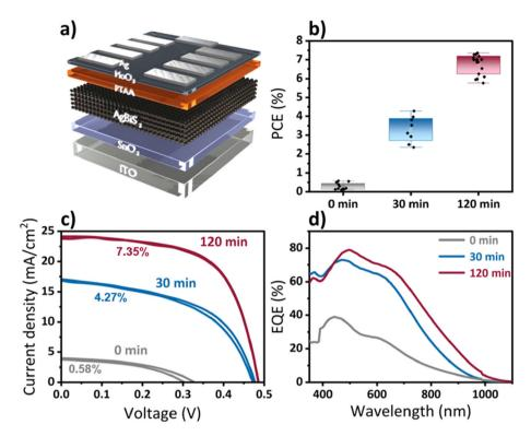
Fig. 5 (a) Schematic device architecture of AgBiS<sub>2</sub> solar cells, (b) Solar cell performance (PCE) of AgBiS<sub>2</sub> QDs obtained after different times of cation exchange, (c) J-V curves (forward and reverse scanning) of devices with different QDs after 0 min (Aq<sub>2</sub>S), and AqBiS<sub>2</sub> after 30 min, and 120 minutes of cation exchange with individual PCE (d) corresponding EQE curves for these three devices.
