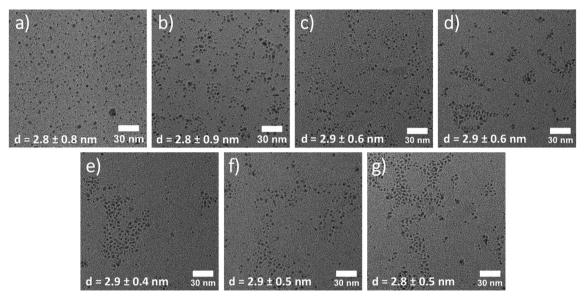
Fig. 2 TEM images of (a) Ag<sub>2</sub>S QDs before and during the cation exchange at (b) 5 min, (c) 15 min, (d) 30 min, (e) 50 min, (f) 80 min, and (g) 120 min of reaction time. Scale bar 30 nm (bottom right) and average QD size and standard deviation (bottom left) for each image.
