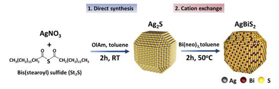
Fig. 1 Schematic representation of Aq<sub>2</sub>S QDs synthesis and formation of AqBiS<sub>2</sub> via cation exchange at mild temperature.
