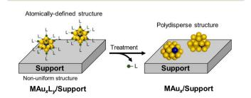
**Scheme 4** Schematic of the synthetic method of SAD Au NCs on a solid support.
