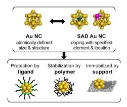
Scheme 1 Pure vs. single-atom-doped (SAD) Au NC.
