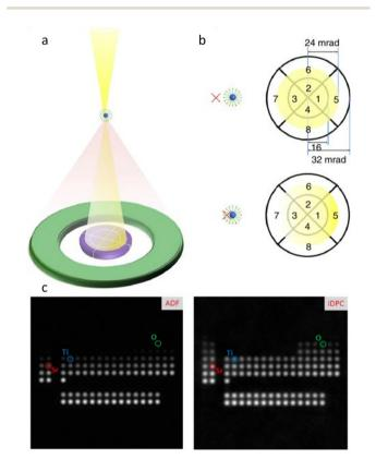
Fig. 5 The schematic illustration and imaging of the segment detector. (a) Segment detector inserted in the bright-field region and (b) intensity distribution for distinct probe position. Reproduced with permission.<sup>51</sup> Copyright 2017, Springer Nature. (c) Simulated ADF-STEM and iDPC-STEM images of the periodic table of elements. Reproduced with permission. 52 Copyright 2016, Oxford University Press.
