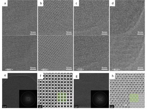
Fig. 10 The low-dose HRTEM images of MOFs. (a)-(d) The raw (top) and denoised (bottom) images of UiO-66 from different zone axes. (e) Driftcorrected, and (f) CTF-corrected and Wiener-filtered images of ZIF-8. (g) Drift-corrected, and (h) CTF-corrected and Wiener-filtered images of HKUST-1. Reproduced with permission. 41 Copyright 2018, The American Association for the Advancement of Science.
