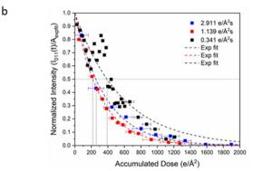
Fig. 3 The effect of total dose on the crystallinity of MOFs. (a) Electron diffraction pattern of ZIF-8 at a dose rate of 0.34 e  $\rm {\AA}^{-2}~\rm s^{-1}$ . (b) The intensities decrease at three different dose rates. Reproduced with permission.<sup>26</sup> Copyright 2019, Oxford University Press.
