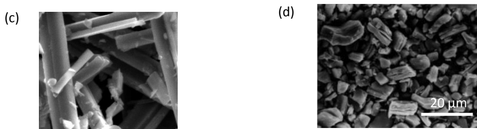
Figure 5. (a) Crystal structure of fibrous-like titanate (monoclinic) 72 ; (b) Crystal structure of lepidocrocite-like titanate (orthorhombic) viewed down along the a-axis 73 ; (c) FESEM image of fibrous-like titanate 73 ; (d) FESEM image of lepidocrocite-like titanate 74 . Panel (a) adapted with permission. 72 Copyright © 2010, American Chemical Society. Panel (b, c) adapted with permission. 73 Copyright © 1995, American Chemical Society. Panel (d) adapted with permission. 74 Copyright © 1998, American Chemical Society.
