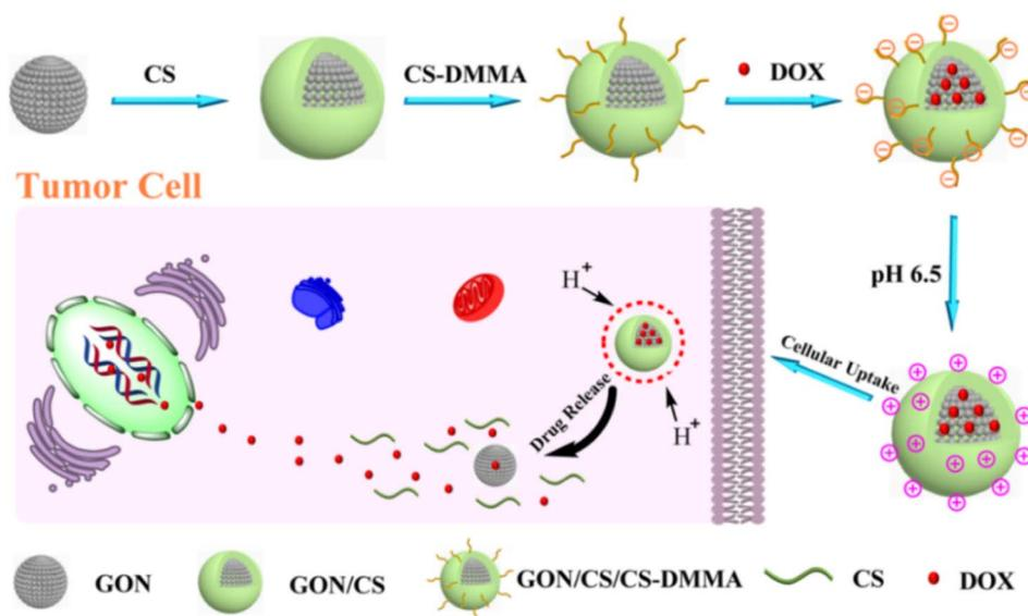
Fig. 6 Schematic illustration of the fabrication and drug release of the GON/CS/CS-DMMA by pH trigger. Reprinted with permission from "X. Zhao *et al.*, "Design and development of graphene oxide nanoparticle/chitosan hybrids showing pH-sensitive surface charge-reversible ability for efficient intracellular doxorubicin delivery," *ACS Appl. Mater. Interfaces*, vol. 10, no. 7, pp. 6608–6617, 2018, doi: <https://doi.org/10.1021/acsami.7b16910>. Copyright–2023–American Chemical Society.
