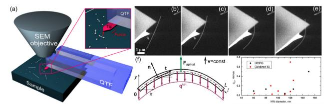
Fig. 14 (a) Experimental scheme of the nanomanipulation of NW with AFM tip glued inside the AFM tip QTF inside the SEM. Reproduced with permission. 198 Copyright 2015, IOP. (b-e) SEM images of a ZnO NW on the HOPG pushed to slide by the AFM tip from the initial to final shape. (f) Mechanical model for calculating the kinetic frictional force on the NW, and kinetic frictions measured as a function of NW diameter on HOPG and oxidized Si wafer. Reproduced with permission. 197 Copyright 2012, Wiley.
