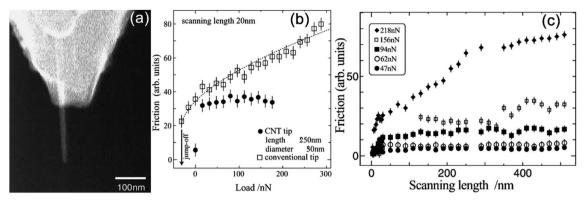
Fig. 7 (a) MWCNT attached to AFM tip. (b) Friction *versus* load curves for both conventional and CNT probes were generated through the analysis of a scanning length set at 20 nm. (c) Friction and scanning length relationship diagram at various applied loads. Reproduced with permission. Elsevier.
