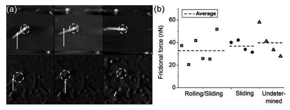
Fig. 6 (a) AFM images of the translation motion of ZnO NW during manipulation when both pure sliding and rolling sliding. The arrow indicates the motion of the probe tip, while the dotted circle indicates the marker on the NW used to assess the degree of rolling. (b) Average dynamic frictional forces measured during the manipulation. Reproduced with permission. <sup>138</sup> Copyright 2013, RSC.
