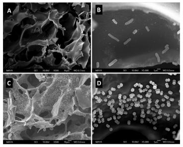
Fig. 16 SEM images of multiple boronic acid ligands containing cryogels with bound *E. coli* (A) and (B) and *S. epidermidis* (C) and (D) on. The scale bars are 10  $\mu$ m in (A) and (C) and 1  $\mu$ m in (B) and (D). Reproduced under terms of the CC-BY license with permission. <sup>58</sup> Copyright 2022, The Authors, published by the American Chemical Society.
