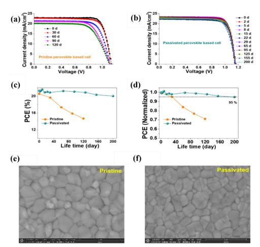
Fig. 5 Comparison of long-term stability (a) and (b) J-V curves, (c) the value of PCEs, and (d) normalized PCE for pristine and PMMA-passivated perovskite solar cells for storage under N2 conditions (25–30% temperature). Top-view SEM images of (e) pristine and (f) passivated perovskite films. Reproduced with permission.  $^{108}$  Copyright 2022, Elsevier B.V.
