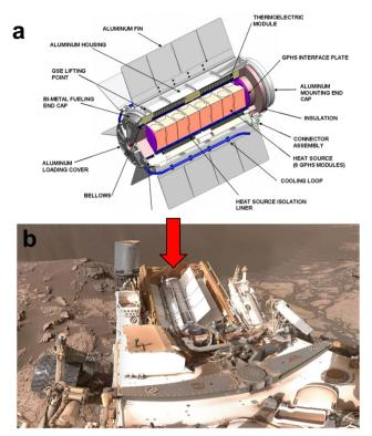
(a) Configuration of the multi-mission radioisotope thermoelectric generator (MMRTG); (b) MMRTG deployed on the curiosity rover during its Mars mission. These figures were redrawn by the authors based on the original figures<sup>21</sup> (Image credit: NASA/JPL/Caltech).
