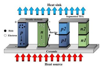
Fig. 1 Thermoelectric (TE) couples, composed of p-type and n-type materials, are connected by metallic electrodes arranged in a series with a  $\pi$ -shaped configuration. A traditional module (left-handed figure) has only one material in a singular leg, while the segmented TE (right-handed figure) module is characterized by the integration of two different materials.
