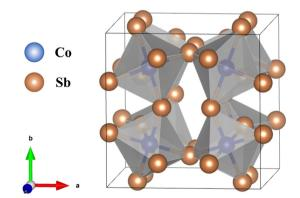
Fig. 11 Illustration of the crystal structure of the  $CoSb_3$ -based alloy, which crystallizes into octahedrons within the space group  $Im\bar{3}$ . The structure is characterized by a void at the center of the cubic lattice. Crystal structure information was sourced from materialproject.org and visually represented using VESTA.<sup>48</sup>
