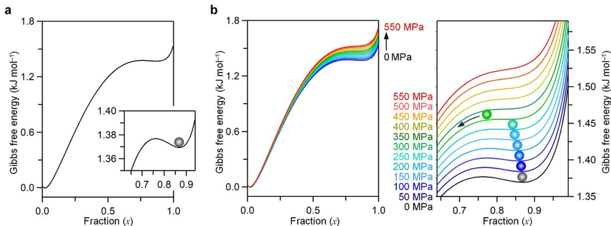
Fig. 5 (a) Gibbs free energy versus fraction curve at 300 K for pressure of 0. Ball indicates the thermal population.  $\lambda$ -Ti<sub>3</sub>O<sub>5</sub> cannot transit to  $\beta$ -Ti<sub>3</sub>O<sub>5</sub> since the energy barrier exists. (b) Pressure dependence of Gibbs free energy versus fraction curves.  $\lambda$ -Ti<sub>3</sub>O<sub>5</sub> transits to  $\beta$ -Ti<sub>3</sub>O<sub>5</sub> by applying pressure because the energy barrier disappears.
