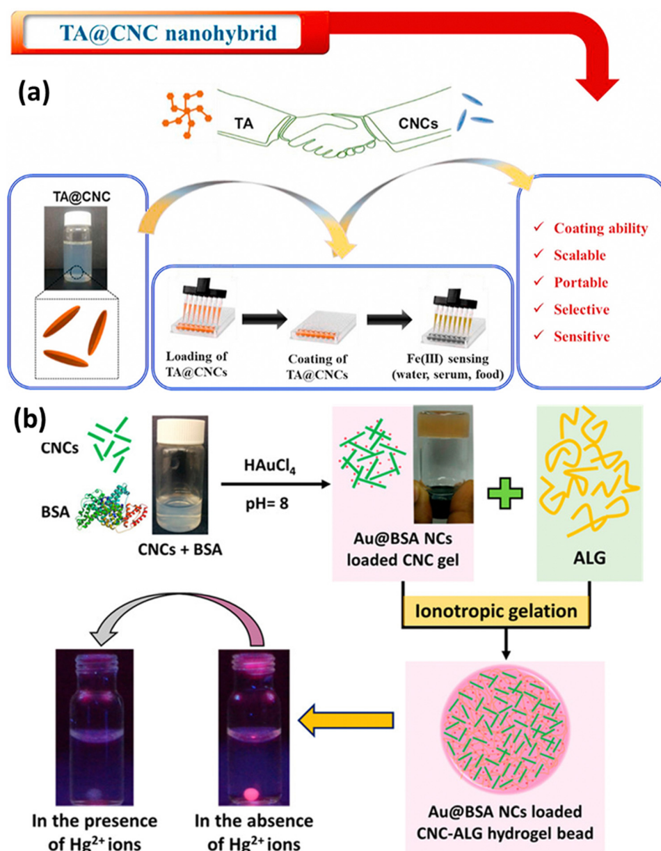
Fig. 5 Use of CNCs in metal sensing: (a) tannic acid loaded CNCs for \text{Fe}^{3+} detection 161 and (b) bovine serum albumin-protected-gold-nanocluster (Au@BSA NC) loaded CNCs–alginate hydrogel beads. 162 Reproduced from ref. 161 with permission from Elsevier, copyright 2021. Reproduced from ref. 162 with permission from ACS, copyright 2016.
