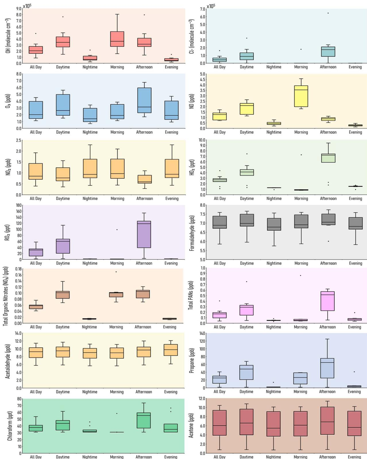
**Fig. 3** Concentrations of key indoor species from ten different houses, showing the median, the upper (75%) and lower (25%) percentiles and the upper ( $Q3 + 1.5 \times IQR$ ) and lower whiskers ( $Q1 - 1.5 \times IQR$ ). The small circles represent values which lie outside of the upper and lower whisker range. The denoted time periods are: all day (12am to 12am), daytime (7am to 7pm), nighttime (7pm to 7am), morning (6am to 12pm), afternoon (12pm to 6pm) and evening (6pm to 10pm).
