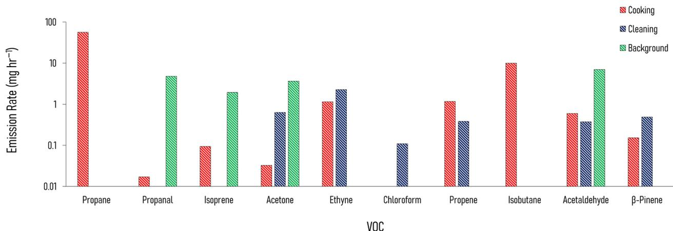
Fig. 4 The enhancement in emission rates from indoors to outdoors over background values for a variety of VOCs ( $\text{mg h}^{-1}$ ) during cooking and cleaning, from the house described in Section 2.4.1. The background emission rates are shown for comparison, and comprise of emissions from building and furnishing materials and from people.
