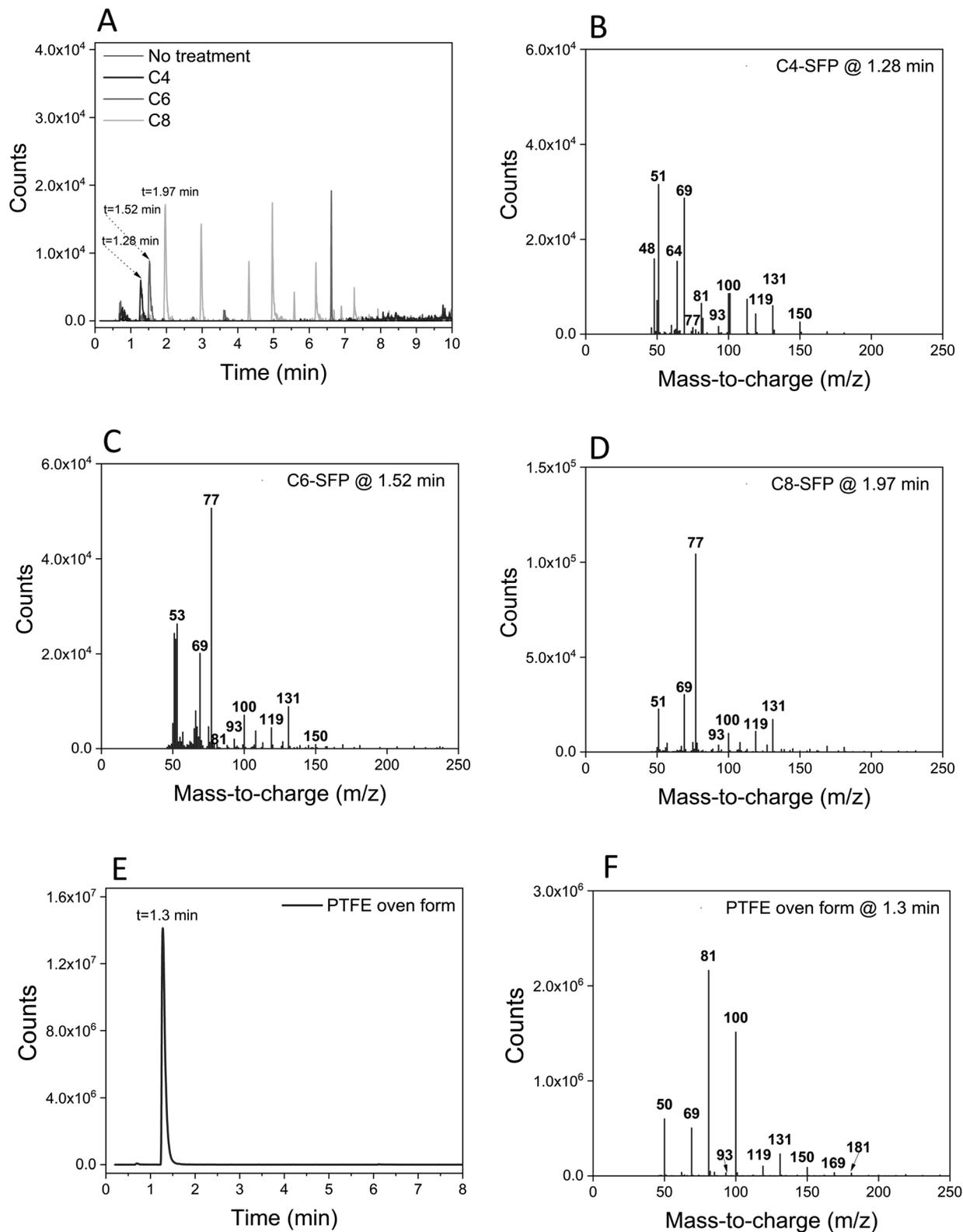
Fig. 2 Extracted ion chromatograms ( $m/z$  131) for C4, C6, and C8 reference textiles (panel (A)) and the associated mass spectra for the first peak in each chromatogram (panels (B)–(D)). Panel (E) shows the total ion chromatogram for the PTFE-coated oven form, while the mass spectrum associated with the single peak at 1.3 min is provided in panel (F).
