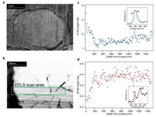
Fig. 4 (a) Cross-sectional scanning electron microscopy (secondary electron detection) of LiNiO<sub>2</sub> particle from an electrode charged to 4.8 V. (b) Selected STEM-EELS scan area of 1.5 μm from surface to bulk (left to right) of the particle. (c) and (d) Fitted peak ratios of depth-resolved Ni L<sub>3</sub>- and O K-edge EELS spectra using a simplified two peak fit in each case (see ESI,† Fig. S11). Insets: Examples of EELS spectra.
