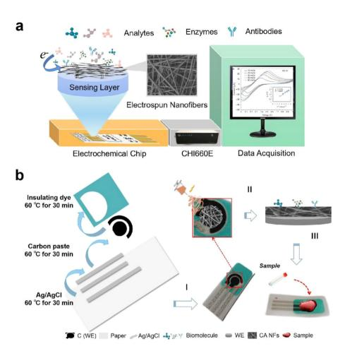
Fig. 1 (a) Schematic of electrochemical biosensor devices based on electrospun nanofibers and (b) the preparation process of the CA NF-decorated PBSP electrode.
