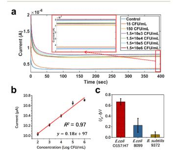
Fig. 6 Performance of the CA NF-decorated PBSP sensor in detecting bacteria. (a) I-t curves and (b) the calibration curve of E. Coli O157:H7 detection; (c) specificity evaluation (compared with E. coli ATCC8099 and Bacillus subtilis ATCC9372).
