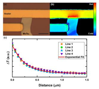
Fig. 4 (a) Optical image of the MoTe<sub>2</sub> device for thermal transport measurement. The scale bar is 5  $\mu m$ . (b) Thermoreflectance map of the sample surface with 5 V supplied to the heater. Temperature decay curves were taken along the sample perpendicular to the heater. (c) Temperature decay curves and their corresponding exponential fit for thermal conductivity extraction.
