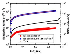
Fig. 3 Scattering rates and DOS as a function of the energy relative to the conduction band minimum  $(E_C)$
