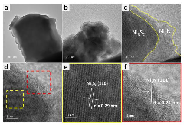
Fig. 3 (a and b) The TEM images of 2-D nanosheets showing the heterostructure of Ni<sub>3</sub>S<sub>2</sub>-Ni<sub>3</sub>N. (c and d) The HRTEM images of Ni<sub>3</sub>S<sub>2</sub>-Ni<sub>3</sub>N showing the formation of an interface between  $Ni_3S_2$  and  $Ni_3N$ . (e and f) The HRTEM images showing the presence of  $Ni_3S_2$  and  $Ni_3N$  phases with the corresponding fringe widths.
