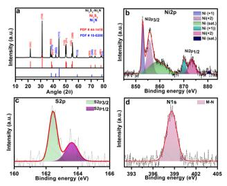
Fig. 1 (a) The PXRD pattern of Ni<sub>3</sub>S<sub>2</sub>-Ni<sub>3</sub>N and (b) the high resolution XPS spectra of Ni 2p, (c) S 2p and (d) N 1s present in Ni<sub>3</sub>S<sub>2</sub>-Ni<sub>3</sub>N.
