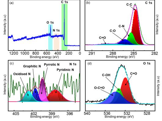
Fig. 3 (a) XPS survey spectrum and (b-d) deconvoluted scan profiles of C 1s, N 1s, and O 1s peaks recorded for the AVAC sample.
