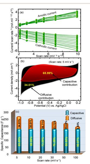
Fig. 6 (a) Linear plots of peak current vs. square root of the scan rate for the cathodic and anodic sweep at different potentials (b) deconvoluted CV profile at a scan rate of 5 mV s<sup>-1</sup> marked with capacitive and diffusive contribution percentages and (c) percentages capacitive and diffusive contributions obtained by Dunn's method for the AVAC electrode.
