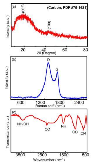
Fig. 1 (a) XRD pattern, (b) Raman spectrum, and (c) FT-IR spectrum recorded for the avocado seed biomass-derived activated carbon.
