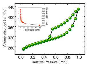
Fig. 4 N<sub>2</sub> adsorption-desorption isotherm curve. Inset: BJH pore size distribution recorded for the AVAC sample.
