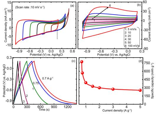
Fig. 5 (a) Cyclic voltammograms at different potential windows at a scan rate of 10 mV s<sup>-1</sup>, (b) cyclic voltammograms at different scan rates, (c) galvanostatic charge-discharge profiles at different currents, and (d) dependence of specific capacitance on the current densities recorded for the AVAC electrode in 1 M KOH in a three electrode cell
