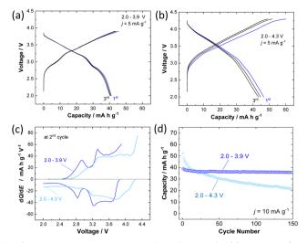
Fig. 2 Electrochemical properties of  $K_{0.6}Cr_{0.6}Ti_{0.4}O_2$ ; (a) the charge/discharge curves of the sample in the potential window range of 2.0-3.9 V at a current rate of 5 mA g<sup>-1</sup>, (b) charge/discharge profiles in the potential window range of 2.0-4.3 V, (c) dQ/dE plots at the 2nd cycle in the voltage range of 2.0-3.9~V and 2.0-4.3~V, and (d) capacity retention for 150 cycles with two distinct voltage cutoffs at a current rate of 10 mA g<sup>-1</sup>.
