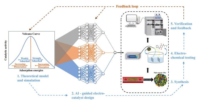
Fig. 1 Proposed Al-guided electrocatalytic decomposition strategy for POPs. Al could accelerate the overall design-synthesis—test cycle by facilitating the theoretical modeling, simulation, design, synthesis, and optimization processes for an optimized electrocatalyst. Given the experimental data of synthesized electrocatalysts, the Al-driven models will be in a continuous iterative upgrade.
