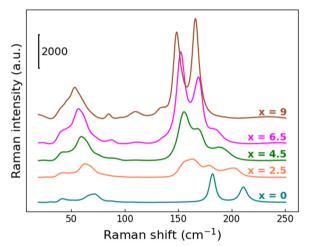
Fig. 9 RT Raman spectra in the region between 25 and 250 cm<sup>-1</sup> for  $Cs_3Sb_2Br_{9-x}I_x$  solid solutions as a function of x.
