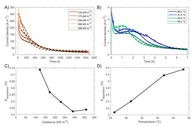
Fig. 7 Results of the model for prediction of BiVO<sub>4</sub> degradation. Experimental and predicted photocurrent densities at (A) different irradiances,  $122-358 \text{ kW m}^{-2}$ , and (B) different temperatures  $26-48 \,^{\circ}\text{C}$ , under  $1 \, \text{sun} = 1 \, \text{kW m}^{-2}$ . (C) Estimated fraction of current towards degradation viadissolution of BiVO<sub>4</sub> as a function of (C) irradiance and (D) temperature.
