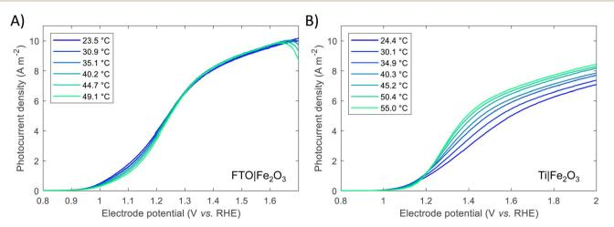
Temperature dependence of voltammograms for (A) FTO|Fe<sub>2</sub>O<sub>3</sub> and (B) Ti|Fe<sub>2</sub>O<sub>3</sub>. Further details are found in the ESI in Fig. S21 and S22.†
