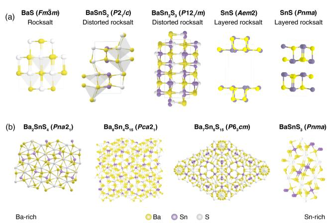
Fig. 4 Experimentally observed crystal structures in the Ba-Sn-S phase space, as well as the predicted thermodynamically stable BaSnS<sub>2</sub> ( $P2_1/c$ ) phase. (a) Rocksalt-derived crystal structures. (b) More structurally complex crystal structures observed experimentally upon annealing.
