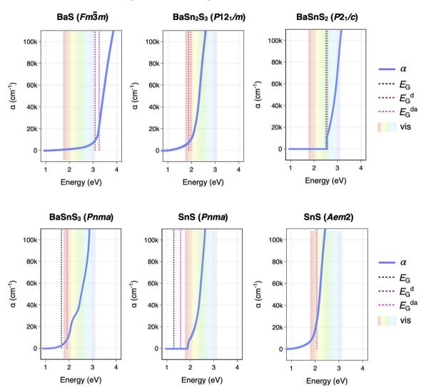
Fig. 6 Computed absorption coefficient for representative Ba-Sn-S phases, plotted in blue. The band gap  $E_G$  is plotted in black, the direct gap  $E_G^d$  in dark purple, and the direct allowed gap  $E_G^d$  in light purple.
