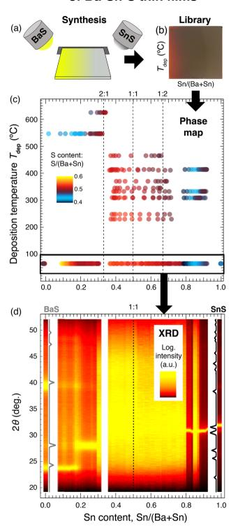
Fig. 1 (a) Deposition setup, (b) a photograph of a combinatorial library, (c) combinatorial phase space of Ba–Sn–S, and (d) XRD heat map of the ambient temperature ( $T_{\rm dep} \approx 60$  °C) region of phase space in (c).
